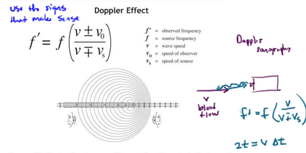
Because of the Doppler effect, the measured frequency of sound is greater for the observer the train is approaching than for the observer the train is leaving.
