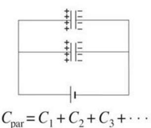
Placing capacitors in series decreases the total capacitance, while placing capacitors in parallel increases the total capacitance.
